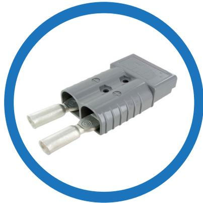
If the battery connector does not match the one on the forklift, contact the battery supplier. Do not make a jumper or alter the existing connectors.
